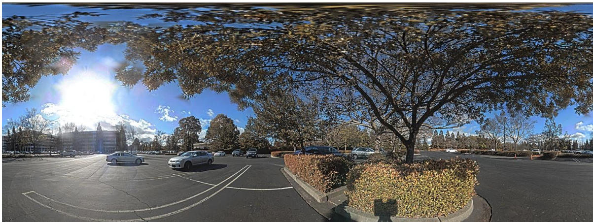
Figure 1: Tone Map image assembly from the Scanstation P40, shown as a spherical projection.
