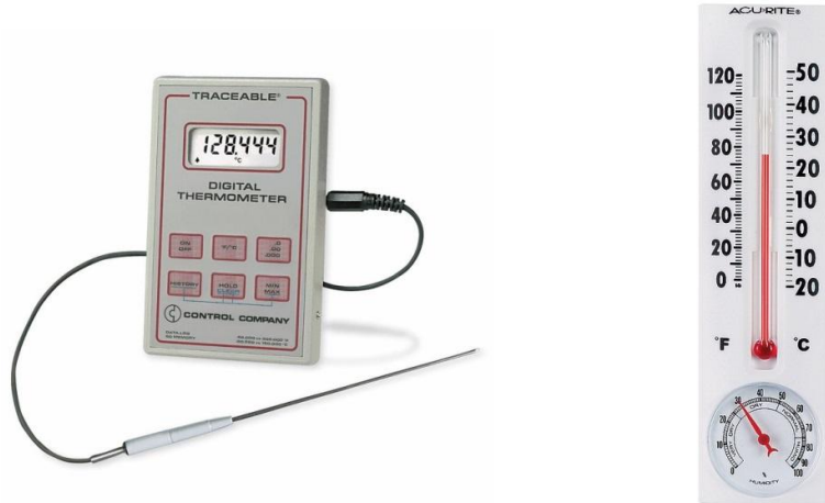
Figure 6: The traceable thermometer on the left is far more expensive than the Acurite® thermometer on the right. The name of the thermometer aside, the uncertainty of the readings on the right are not known explicitly given, because they are likely not known. For the purpose of determining if you need to wear a jacket or not, the uncertainty is not very important.
