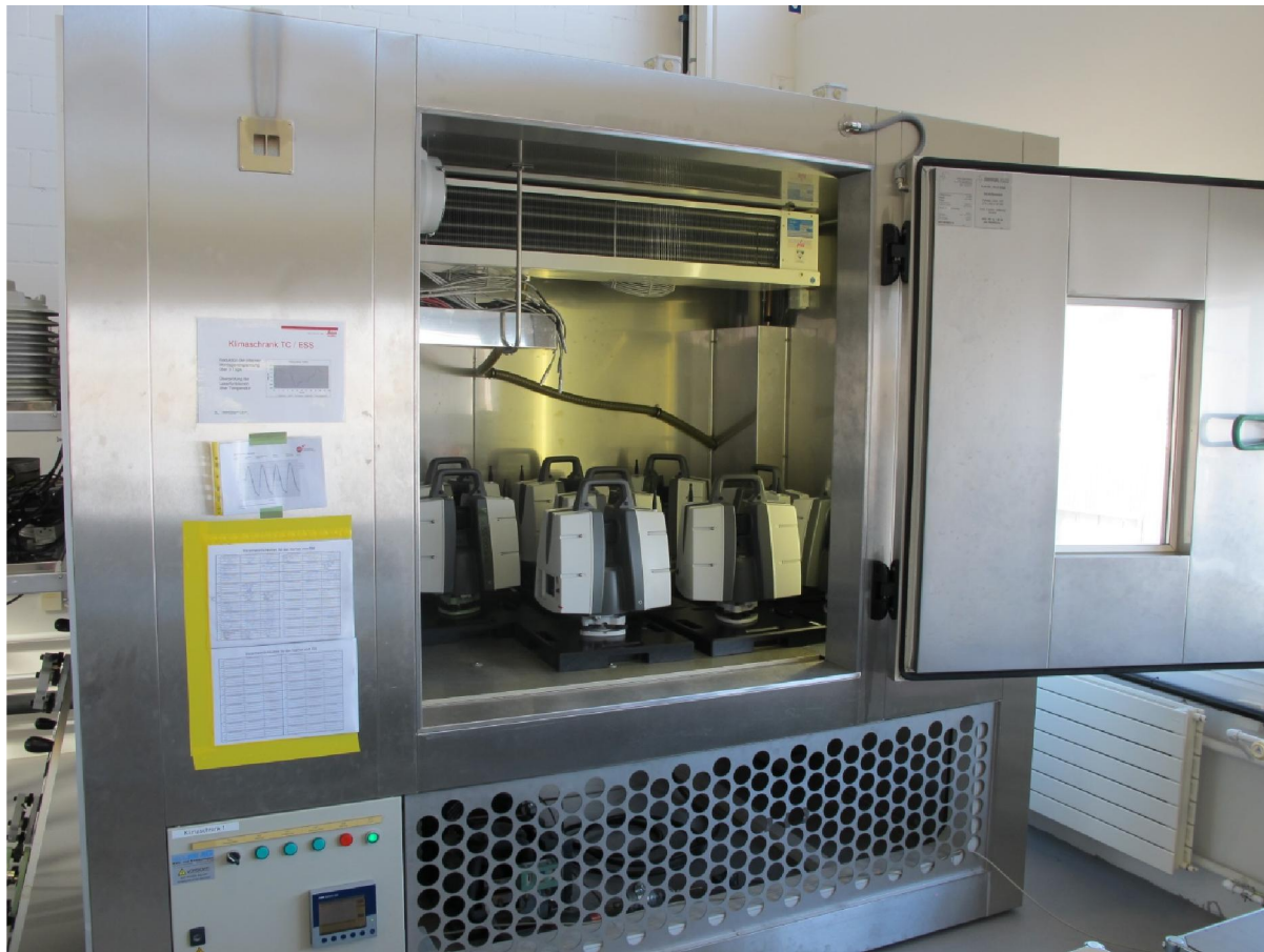
Figure 12: Environmental chamber for thermally cycling P and C series laser scanners. This station is called ESS, or Environmental Stress Screening.
