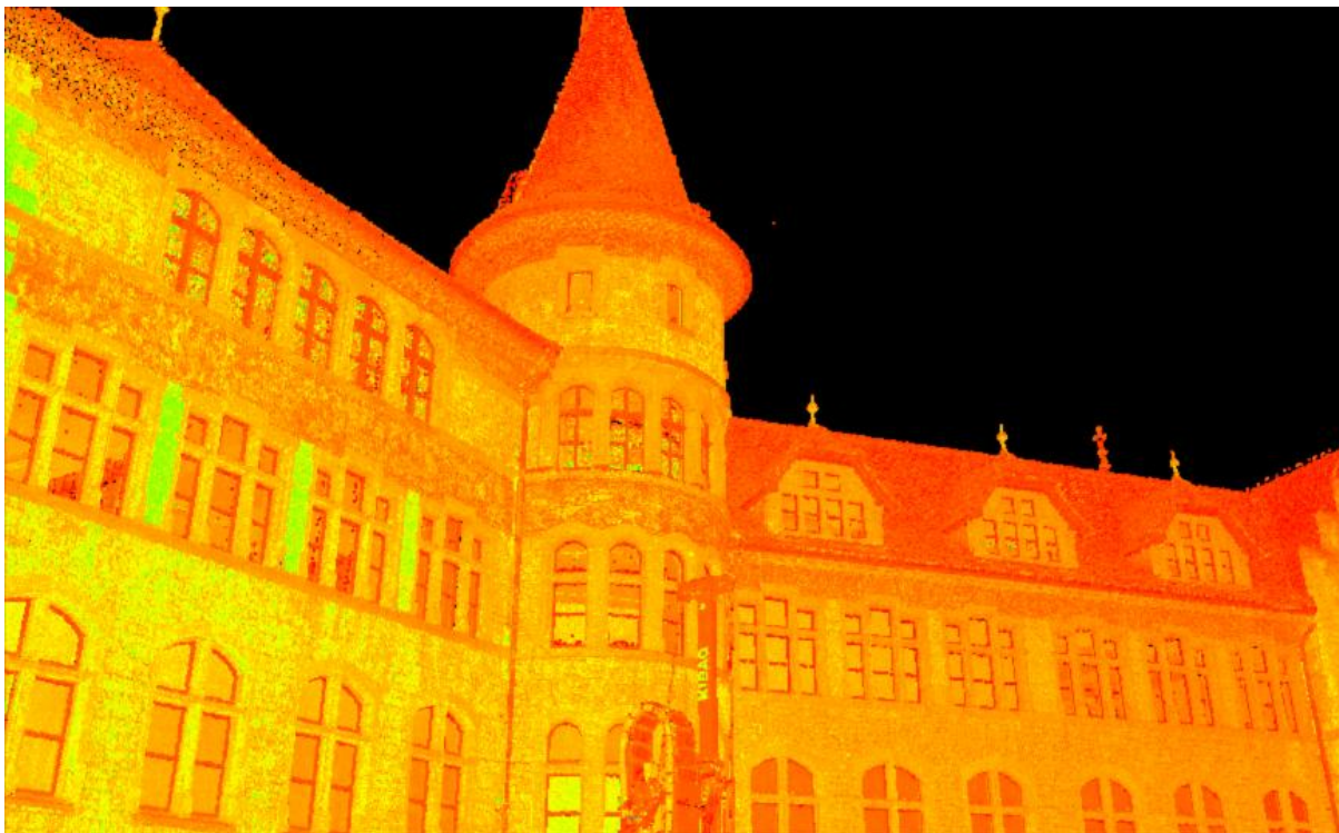
Figure 2: Laser scan of a building provides a lot of detail. Literally this view shows in context millions of measurements.
