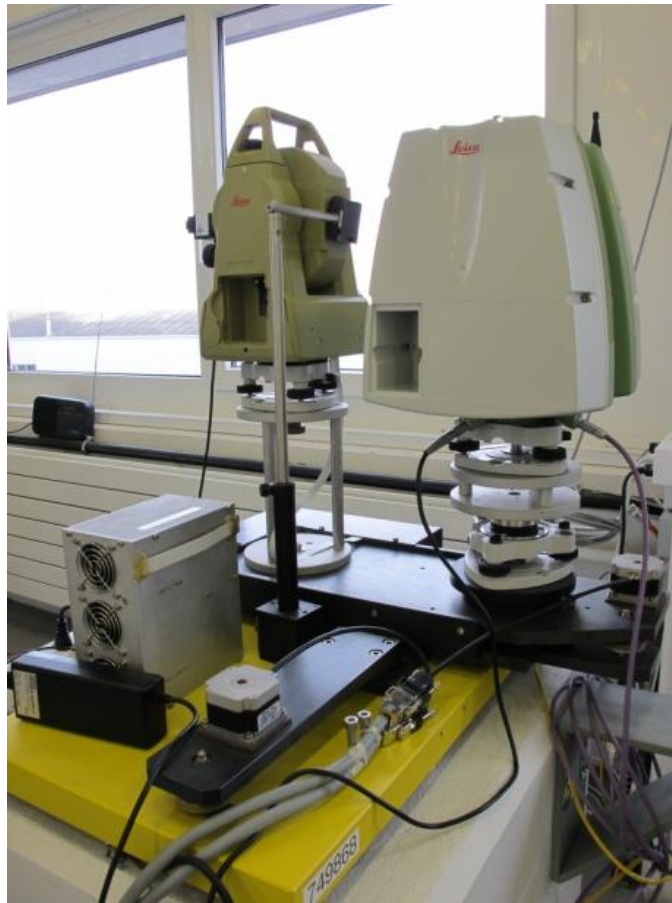
Figure 18: Tilt calibration station for the Leica Scanstation C10. The tilt sensor as it is mounted in the scanner is also observed over temperature.
