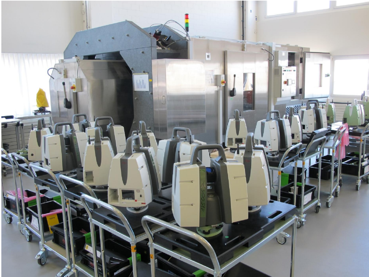
Figure 13: A collection of P40 Scanners waiting for their turn on the ATEC Calibration Rig. To the human eye, they are perfectly identical, but the human eye is not designed to discern microns. To the Antipodal Telescope Environmental Chamber (ATEC), they are all snowflakes.
