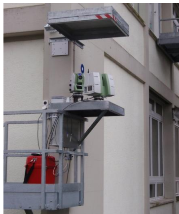
Figure 25: The mounting station for outdoor scanner verification, with a TS30.
