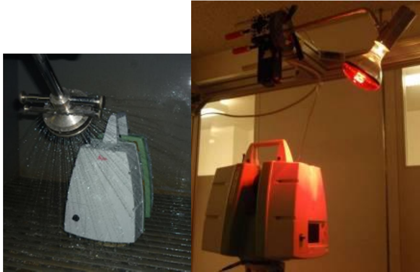
Figure 23: A mosaic of testing events for the C and P series scanners. There is something such as a thing as a regulation shower head, among other things.
