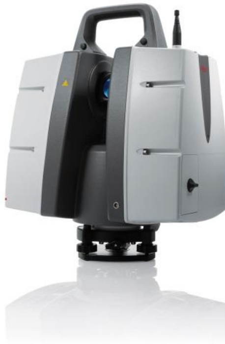
Figure 1: The Leica Scanstation P40, a survey grade laser scanner, with integrated tilt sensor, mounted on a surveying tribach. The tribach has three little wheels to allow fine leveling.
